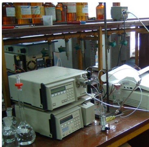
HPLC (high performance liquid chromatography) equipment at the Environmental Chemistry Laboratory.
