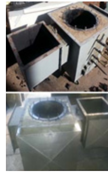
Micro-gasifier stove and Injera baking biomass gasifier and reactor by Dr. Kamil.
